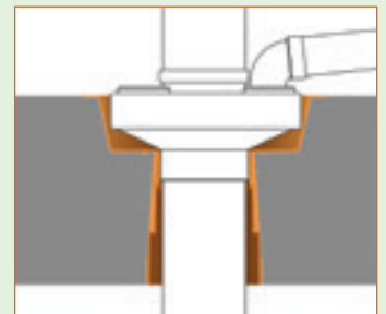
Cross-section of QuelCast Cast In Fire Collar installed with a Manifold on the Top
