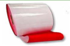
Wraptite 245 Detailing Tape consists of a triple layer polypropylene micro-porous film laminate, with a proprietary acrylic moisture vapour permeable adhesive and silicone-coated PET release liner.
