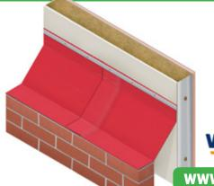
The DPC is a flexible 0.6mm composite damp proof course and cavity tray system. It is supplied in 20m length rolls and the following standard widths: 225mm, 450mm, 500mm, 600mm, 700mm, 800mm and 900mm. Other widths are available on request.
