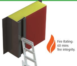
60-minute fire-rated cavity closer for eliminating damp and cold bridging around doors, windows, and sills.
