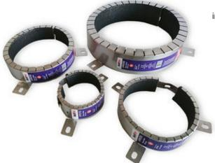
FP170 Intucollar comprises of a stainless steel shell and a reactive intumescent lining. FP170 expands when exposed to fire, reinstating the fire performance of compartment walls and floors which have been penetrated by combustible pipes.
