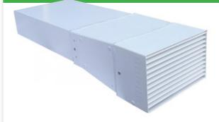
Titon FireSafe® Air Brick Range is a unique high flow terminal designed for powered ventilation systems offering low resistance to airflow, but high resistance to fire as set out in Approved Document B (fire safety) volume 1: Dwellings, 2019 edition. Constructed from sheet steel (A1) and polyester powder coated to classification A2-s1, d0.
