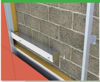
ARC Rainscreen Barrier has been designed to provide a two hour fire rating where continuous vertical airflow is required behind a rainscreen cladding system.
